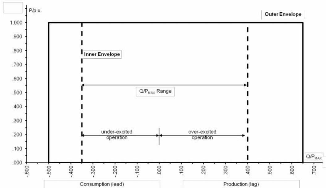
The diagram represents boundaries of a P-Q/Pmax-profile at the connection point by the active power, expressed by the ratio of its actual value and the maximum capacity pu, against the ratio of the reactive power (Q) and the maximum capacity (Pmax). The position, size and shape of the inner envelope are indicative.
