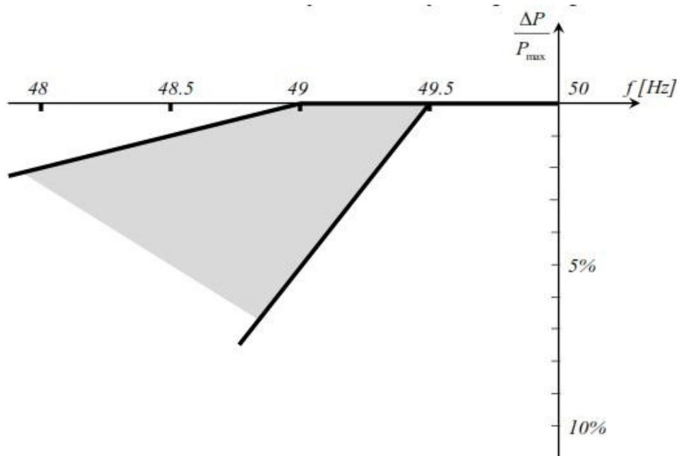
The diagram represents the boundaries in which the capability may be specified by the relevant TSO.
